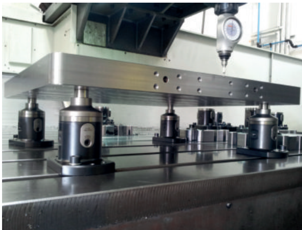
4 basic modules H=100 positioned directly on the machine table. The 4 reducers H=50 on top facilitate optimum access to workpieces. Clamping height 150 mm
