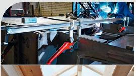
Alongside complete assembled high-performance clamping sets BESSEY also offers versatile accessories that can be combined with one another. Sliding arms that are already fitted can be changed over from clamping to spreading or replaced by different sliding arms or even supplemented with others.
