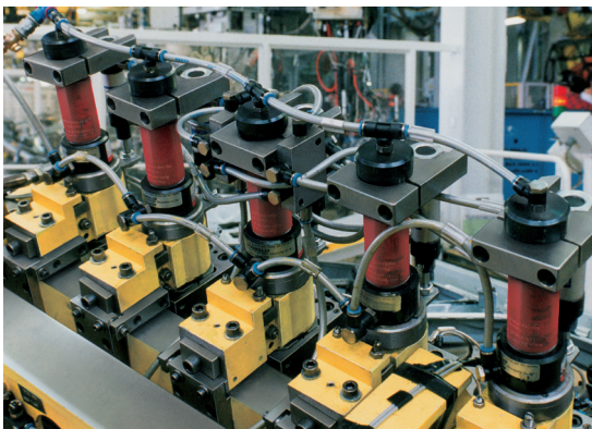
Stamping units placed in line
