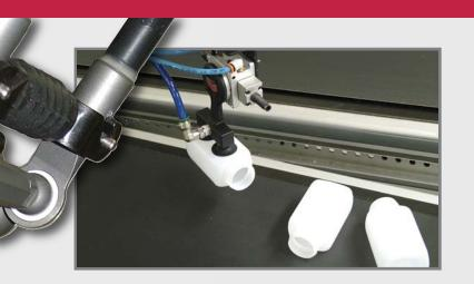
DE-STA-CO's "5th Axis High-Speed Pick and Rotate" is a pneumatically actuated mechanism designed to be applied as a non-programmable, supplemental axis to ABB's IRB 360 Flex-Picker as well as other robotic and fixed automation systems involved in high speed pick and place of small, light weight objects.
