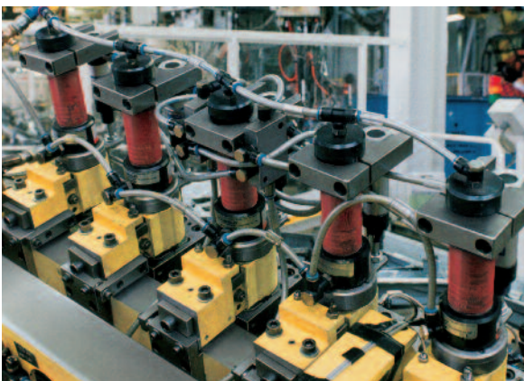
Stamping units placed in line
